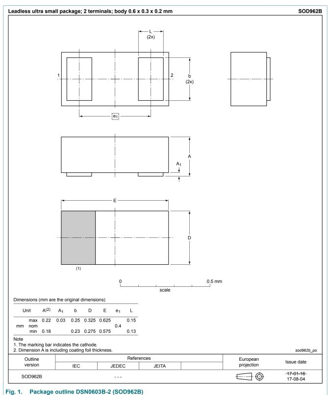
silicon, leadless ultra small package; 2 terminals; 0.4 mm pitch; 0.6 x 0.3 x 0.2 mm body
